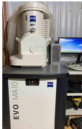
Figure 1. Schematic of SEM - EVO MA 10 (Zeiss, Germany) scanning microscope.
