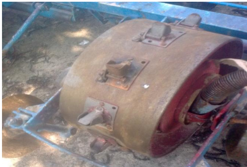
Fig. 5. Corrosion of AN-2 seed drill
