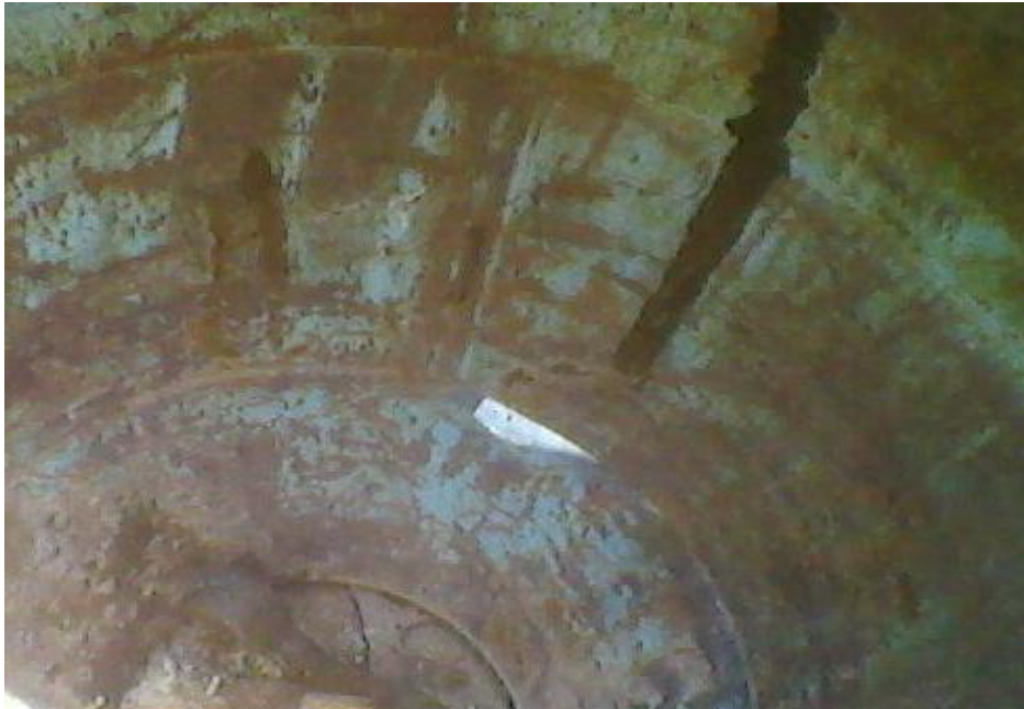
Fig. 8. Rusting of KXU-4 cultivator fertilizer hopper
