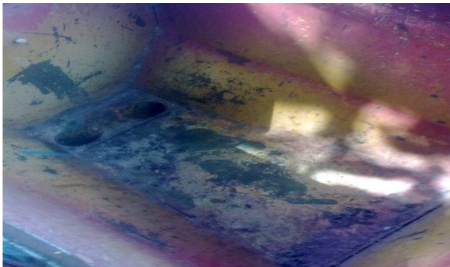
Fig. 2. Rust of AN-2 seed drill
