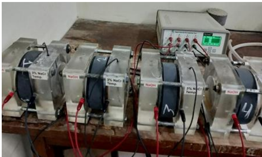
Figure 3: Setup for RCPT Test
