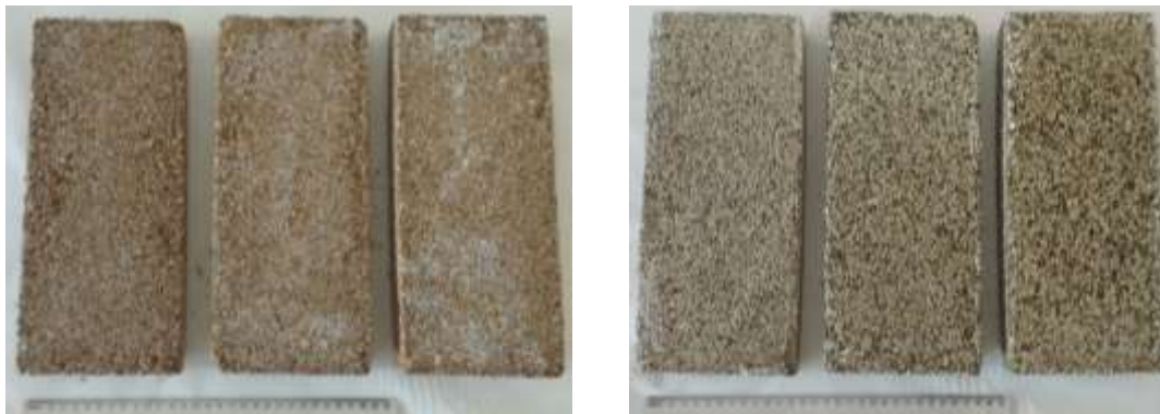
Plates made of thermally expanded vermiculite
