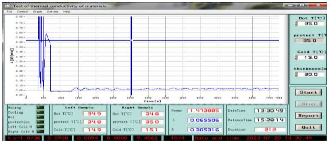
Figure 4. Plate obtained on the basis of expanded vermiculite XND-2-3030 C of sample #1 on the machine the results of determining the heat transfer coefficient
